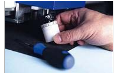
Tool head change with only one tool (included) in less than 1 minute.
